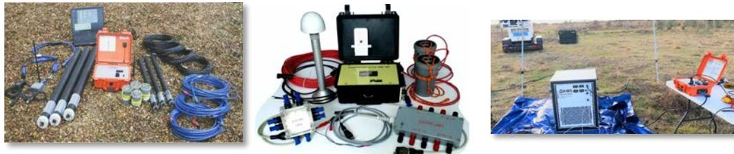
*KMS-200 software works with MT data from KMS-820 MT system (left), LEMI-424 system (middle) or KMS-820 CSEM system (right)*
